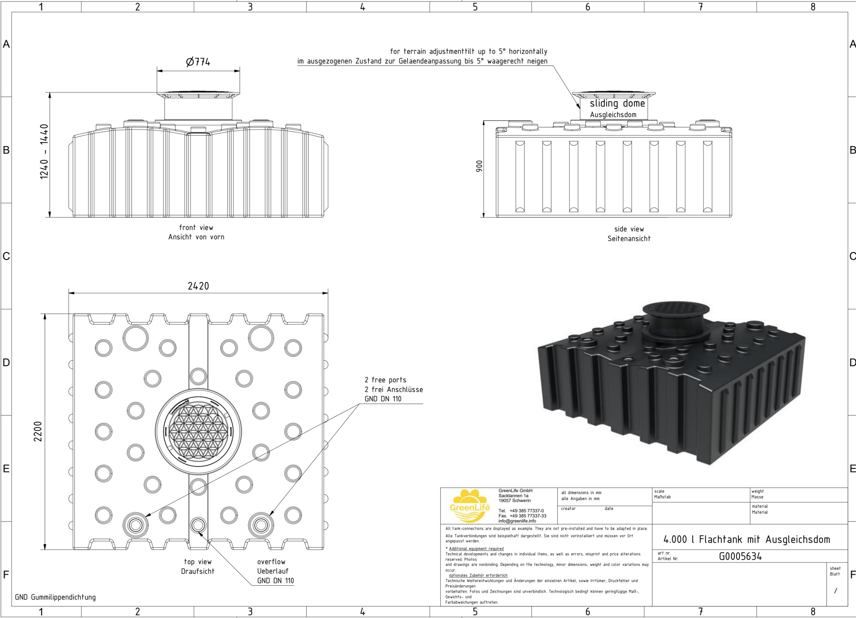
for terrain adjustment tilt up to 5° horizontally
